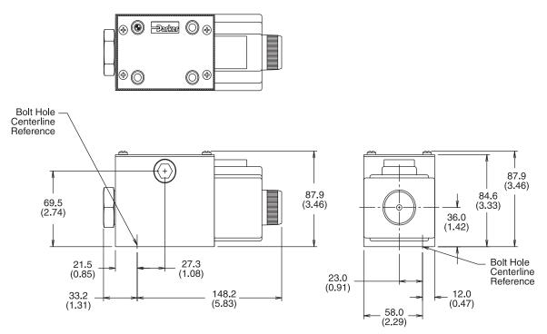
Note: 30 mm (1.18") from bottom of bolt hole counterbore to bottom of valve.
