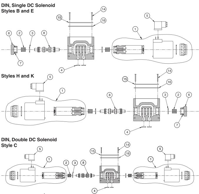
Replacement Parts† DC DIN Solenoid, Styles B,C,E,H,K
