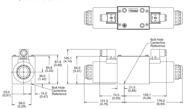
Note: 30 mm (1.18") from bottom of bolt hole counterbore to bottom of valve.
