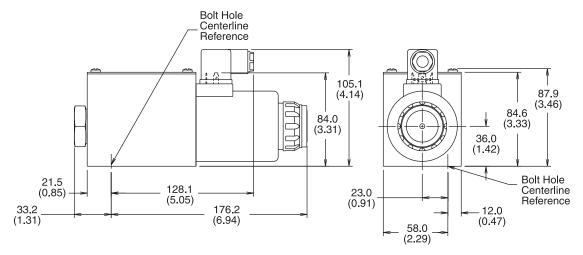
Note: 30 mm (1.18") from bottom of bolt hole counterbore to bottom of valve.
