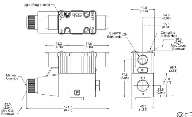
Note: 22.0 mm (0.87") from bottom of bolt hole counterbore to bottom of valve.
