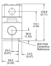
Note: 30 mm (1.18") from bottom of bolt hole counterbore to bottom of valve.
