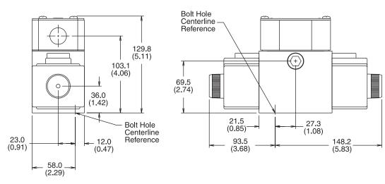
Note: 30 mm (1.18") from bottom of bolt hole counterbore to bottom of valve.
