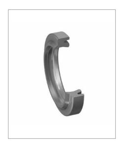
The wear-resistant Ultrathan® AY double wiper ring serves to prevent ingress of dust, dirt, sand and swarf. This is achieved by its special design which largely prevents scoring, protects the guiding parts and extends the service life of the seals. In addition, the sealing lip facing the media side reduces the residual oil film. The AY double wiper ring closes the cylinder vis-à-vis the environment.
