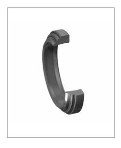
The A1 wiper ring serves to prevent ingress of dust, dirt, sand and swarf. This is achieved by its special design which largely prevents scoring, protects the guiding parts and extends the service life of the seals. An oversized outer diameter ensures interference fit in the groove, thus preventing ingress of foreign particles and moisture via the static seal fit of the wiper.
